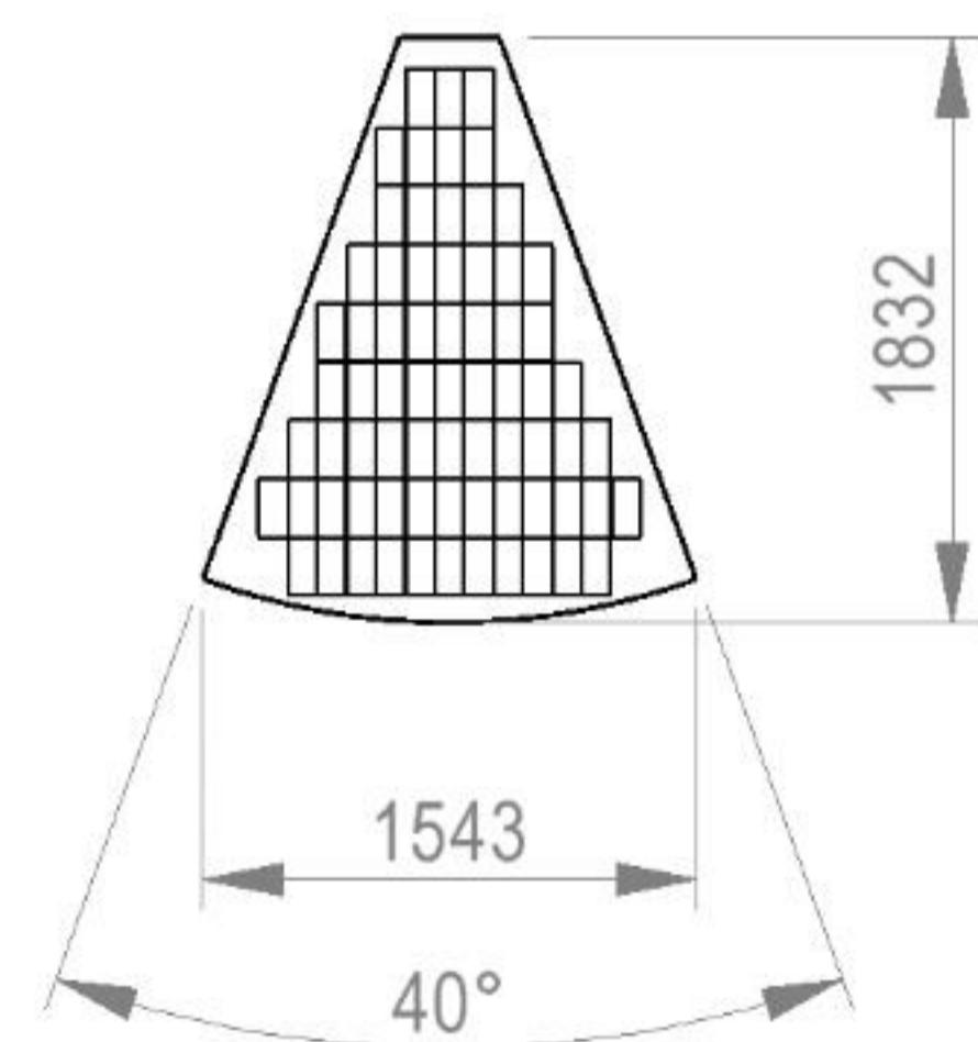
Figure 2. Dimension of solar panel
